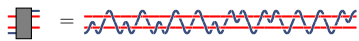
FIG. 4 (color online). An example of an injection weave for the Fibonacci anyon model [ SO(3)_3 or SU(2)_3 ]. This injection was first discussed in Ref. [7] and approximates the identity operation on the Hilbert space to better than one part in 10^2 , while transferring the warp quasiparticle from the bottom to the top. Longer weaves will approximate the identity exponentially more closely with the weave becoming longer only linearly [7,16]. The box on the left establishes the notation used in Fig. 5 below.
