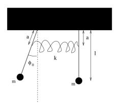
The two pendulums are constrained to swing in the vertical plane passing through both suspension points.
